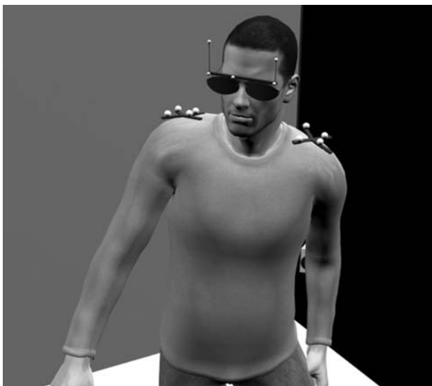
Fig. 3 Representation of the subject's equipment, with markers attached to stereo glasses and a set of markers on each shoulder
